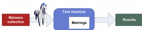
Figure 3: Test arrangement. Trojans were installed one-by-one on a test machine and Mstrings was run. The results were stored in a database.
